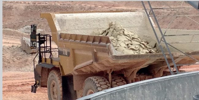
Filterkuchen aus der Gesteinswäsche Filter cake of the washing process of mineral mining
